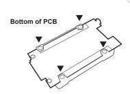
■ Step 4 Turn over the PCB and secure the hard drive to the PCB with the mounting screws that come with the kit.
